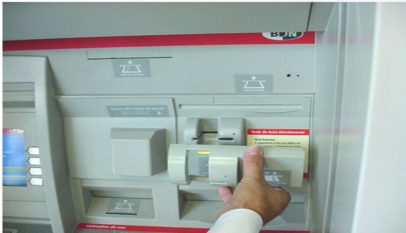
Installing a magnetic card reader attachment
